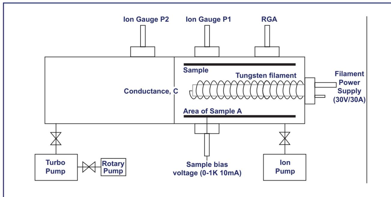
Figure 1. ESD Experimental Arrangement
